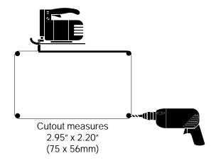
After the panel is drilled and cut, remove all burrs and file down rough edges. Check to make sure that the panel is still flat. Mounting the display on a distorted panel may cause improper operation of the adjustment keys. Install the panel display into the cutout.
