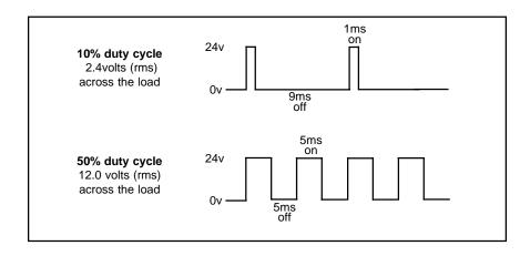
PWM voltage can be measured with a conventional analog meter (the type with a moving pointer). However, a digital DC volt meter should not be used unless it is of a "*true RMS*" type (a feature offered on newer meters). To measure the PWM voltage, connect the voltmeter across the load device.
