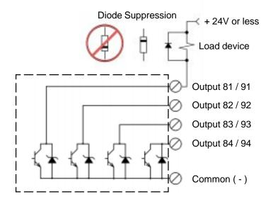
Caution: Exceeding 24 volts or 1/2 amp will damage the output transistor and is not covered under warranty. Therefore; be sure that a 24v load device does not measure less than 48 ohms or a 12v load device does not measure less than 24 ohms. Also be sure that the DC supply used for the loads is of a regulated type that will not exceed 24 volts unloaded. Avoid using switching power supplies that require a minimum load current.
